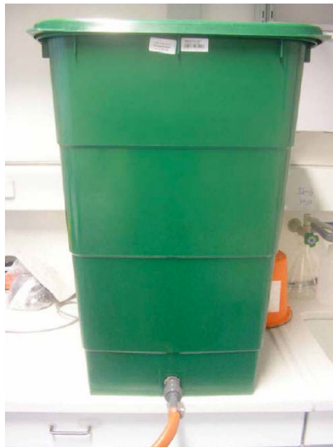
Picture 1: Container used for examining separation of radioactive substances from drinking water
